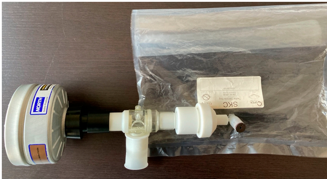
Figure 1. Setup for breath collection. From left to right: A2-environmental VOCs filter; 2-way non rebreathing valve; expiratory port; tedlar bag.
